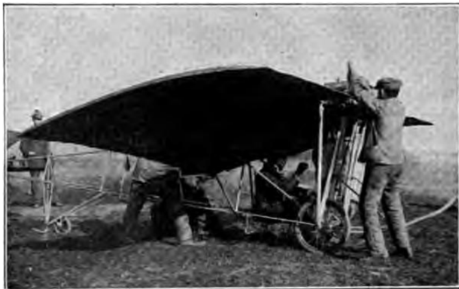
Fig. 22. Method of Starting the Engine of an Aeroplane
